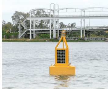
Figure 110. Floating water level and water quality/salinity monitoring Figure 11: Floating water level and water quality/salinity monitoring
