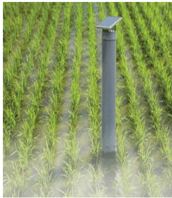
Figure 132. Smart sensor measures water level in rice fields for AWD Figure 13: Smart sensor measures water level in rice fields for AWD
