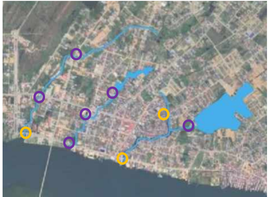
Figure 14 Initial Recommendation for Location of Trashbooms
