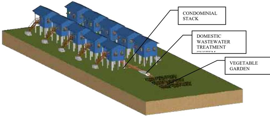
Figure 6 Conceptual perspective for wastewater treatment system for demo house community.
