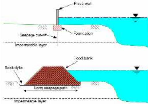
Figure 3 Typical elements of a permanent flood protection system<sup>5</sup>
