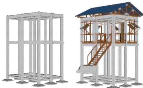
Figure 5 Conceptual base structure for proposed resilient housing design.
