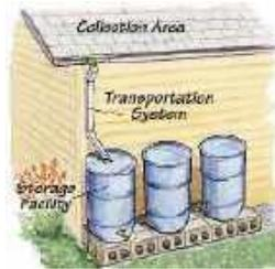
Figure 9 Conceptual diagram for rainwater harvesting system
