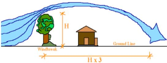
Figure 8 Conceptual diagram for protective vegetation
