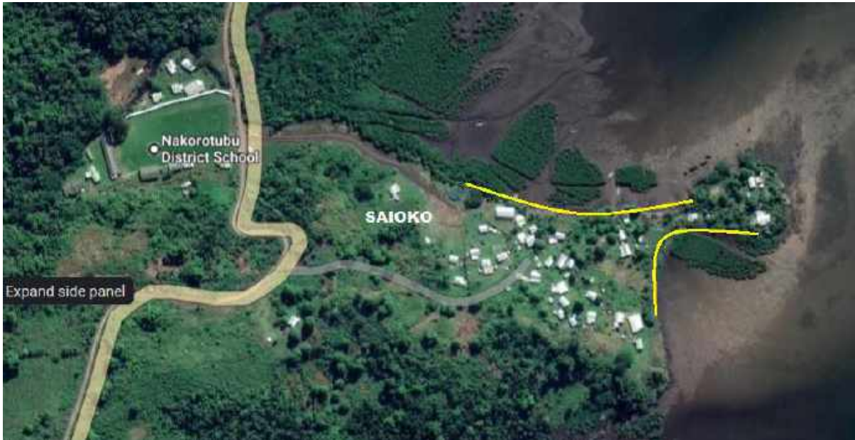
Figure 42 Proposed extent of seawall for Saioko Village.
