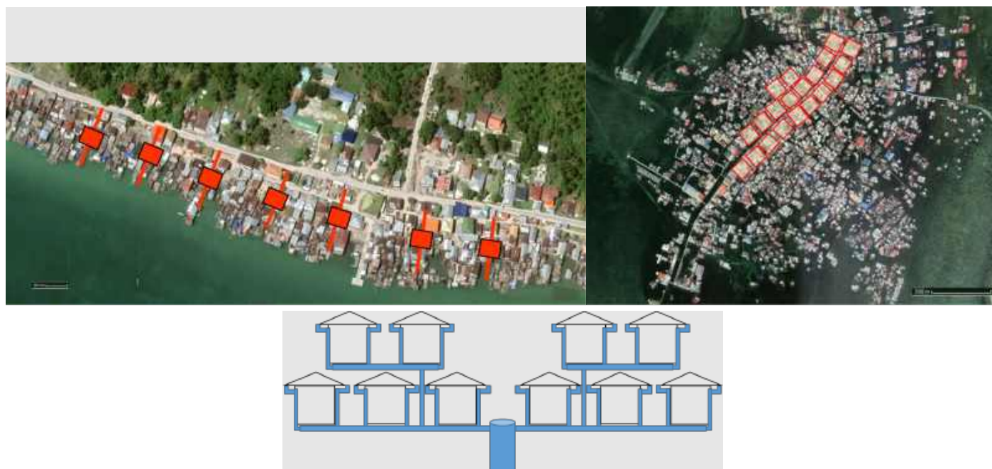
Figure 18. Illustrative example of communal rainwater harvesting clusters
