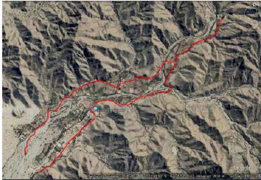
FIGURE 8. IRRIGATION SYSTEM TRUNK PIPING FOR ANTINACO, CATAMARCA
